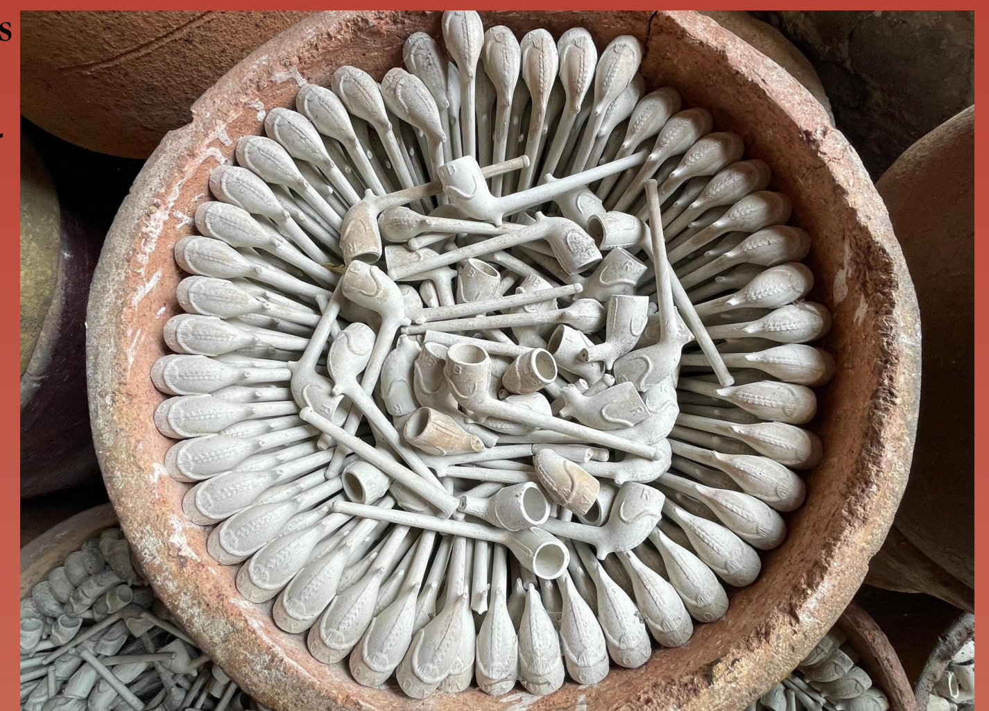
Figure 3. Ceramic saggars protect tobacco pipes during firing (Rack and Tisdale 2024).
